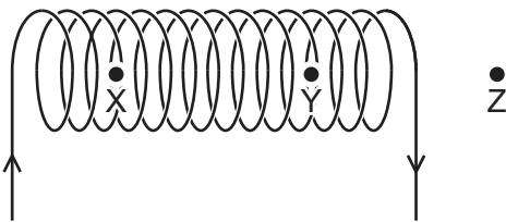
Which row compares the strength of the magnetic field due to the solenoid at points Y and Z with the strength of the magnetic field at point X?
